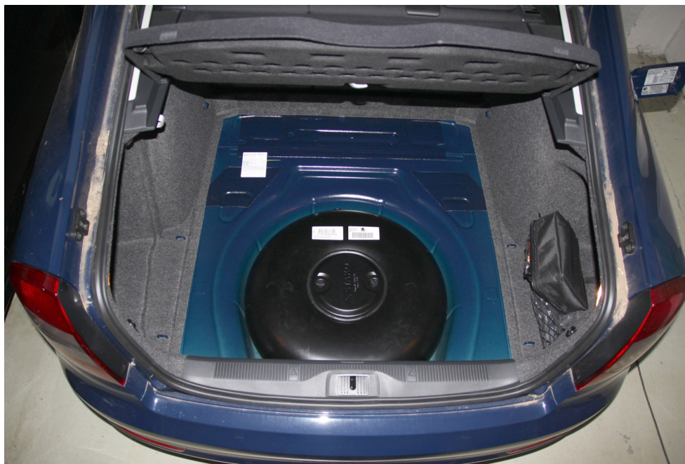
Fig. LPG tank in the spare wheel well under the luggage compartment floor.
