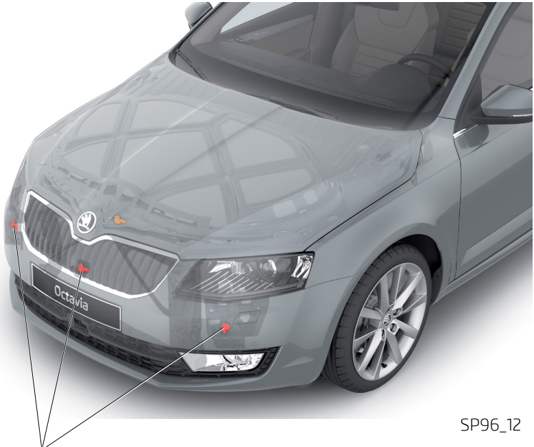
Crash sensors of the pedestrian protection system
